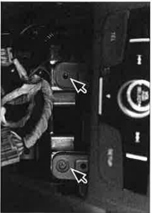
3. Remove both screws (keep screws, they will be needed later)
