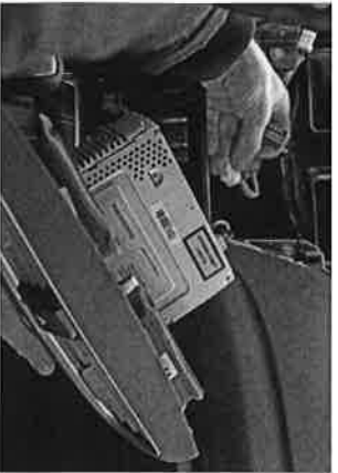
4. Remove OEM head unit by pulling it towards your direction
