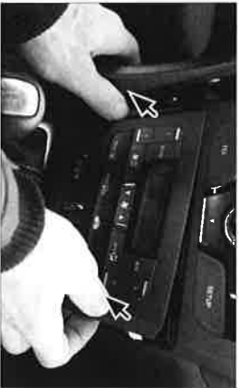
2. Remove air condition control panel (below the radio)
